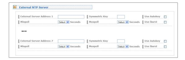
By using the NTP configuration page, a number of additional parameters can be added to this default ntp.conf. In the upper section up to seven external NTP servers can be set up to provide a high grade of redundancy for the internal reference clock. For each of these external NTP servers the AUTOKEY or symmetric key feature of NTP can be used to ensure the authentic of these time sources.
