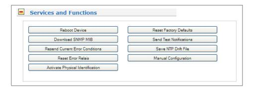
With "Manual configuration" you are able to change the main configuration by editing the configuration file by hand. After editing, press the "Save file" button to preserve your changes, afterwards you are asked if your changes should be activated by reloading the configuration (this results in reloading several subsystems like NTPD, HTTPD etc.).
