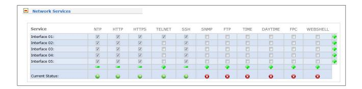
In the second section the possible network protocols and access methods can be configured. You can enable/disable NTP, HTTPS, TELNET, SSH, SNMP, FTP, TIME, DAYTIME, FPC and WEBSHELL by checking/unchecking the appropriate check boxes. After you saved your settings with the "Save Settings" button, all these subsystems are stopped and eventually restarted (if they are enabled).
