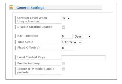
The "Local trusted key" field holds a list of all trusted symmetric keys (comma or space separated), which have to be accepted by the NTPD of your LANTIME.
