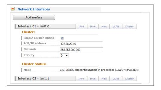
In our example, we will choose the virtual port 01 (assigned to the physical interface LAN 0 of this time server) as cluster port. The cluster tag of this interface is selected and the corresponding fields are filled with the cluster-IP and subnet-mask, as shown in the dialog screen above.
