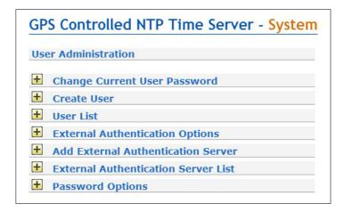
It is possible to create multiple user accounts on a LANTIME system, each account can be assigned one of three access levels: the Super-User level has full read-write access to the configuration of the LANTIME system, it can modify all parameters and has full shell access to the system when logging in via Telnet, SSH or serial console port.
