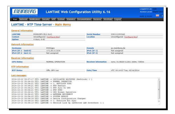
After entering the right password, the main menu page shows up. This page contains an overview of the most important configuration and status parameters for the system.
