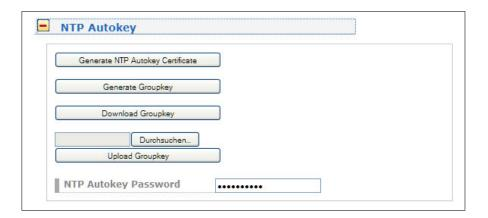
In networks with a lot of clients, this can lead to a logistic problem, because the server key has to be changed on every single client. To help the administrator to reduce this work (or even eliminate it completely), the NTP developers invented the AUTOKEY feature, which works with a combination of group keys and public keys. All NTP clients are able to verify the authentic of the time they received from the NTP servers of their own AUTOKEY group by using this AUTOKEY technique.
