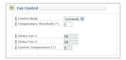
With the optional fan control menu the current status of the operational temperature and the fans can be displayed on the systems interface. The mode of the fans can be selected here:
