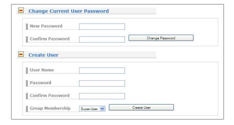
The "User Management" menu allows you to set up different users with password and the access level. To change the properties of an user you have to delete the old user and set up a new one. The user "root" cannot be deleted and has always the membership of Super-User. The password of the user "root" can be set on the security page.
