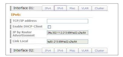
If you enabled the IPv6 protocol, the LANTIME always gets a link local address in the format "fe80:: ....", which is based upon the MAC address of the interface. If a IPv6 router advertiser is available in your network and if you enabled the IPv6 autoconf feature, your LANTIME will be set up with up to three link global addresses automatically.
