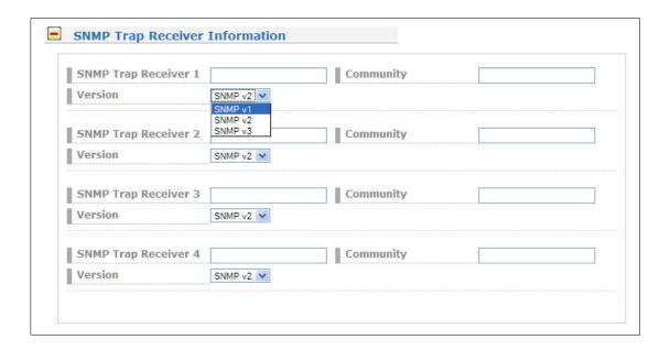
Up to four independent SNMP trap receiver hosts can be configured in this subsection, you may use IPv4 or IPv6 addresses or specify a hostname. Additionally you have to enter a valid SNMP community string for your trap receiving community. These can be unrelated to the SNMP community strings used for status monitoring and configuration access (see SNMP configuration on the "Security" page).
