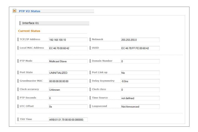
All configuration parameters of the PTP unit can be viewed and changed by accessing the "ptp2\_global\_conf\_0" file. This can be done with the "PTP v2 Configuration" submenu. If more than one PTP unit (PTP ports) is built into the system, then the configuration for each port can be edited separately and will be listed on this page.
