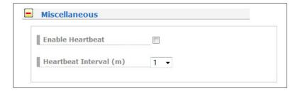
A heartbeat is a periodic signal generated by hardware or software to indicate normal operation or to synchronize other parts of a system. Usually a heartbeat is sent between machines at a regular interval on the order of seconds. If a heartbeat isn't received for a time - usually a few heartbeat intervals - the machine that should have sent the heartbeat is assumed to have failed.
