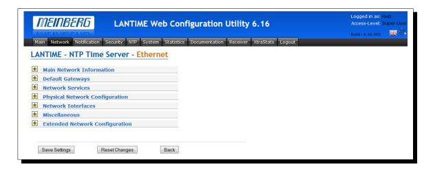
In the network configuration all parameters related to the network interfaces can be changed. In the first section you can edit the hostname and domain name. You can also specify two nameserver - in the nameserver field you may enter an IPv4 or IPv6 address.
