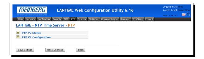
In the PTP section, all parameters of the PTP subsystem can be configured. The current state can be monitored as well. When operating in SLAVE mode (as with MRS devices), a graphical representation of the offset and the path delay to the grandmaster will be shown on page **Statistics** -> **PTPv2 Statistics**.
