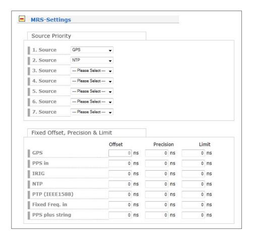
In the next menu the user can define in which order the references will be used to control the internal oscillator. The reference clock with the highest priority will be used always if this is available. You can set an fixed offset for the available references in the next sub menu. By default this value is 0 ns. The bias of the internal GPS receiver can not be set up — indirectly this can be done via the antenna cable length.
