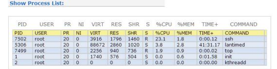
A list of all active processes (CPU performance, used memory, runtime...) of the LAN-CPU is indicated with this table.
