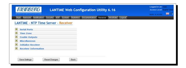
On this page you can edit the important receiver settings like "Serial Ports" or "Time Zone" and you can get an overview about the information of ypur LANTIME's internal receiver.
