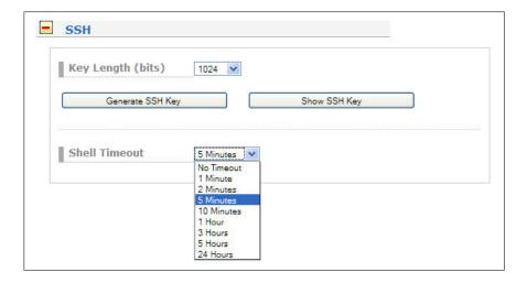
If you enabled SSH, your LANTIME automatically is able to use secure file transfer with SCP or SFTP protocol. The usage of FTP as a file transfer protocol is as insecure as using TELNET for shell access.
