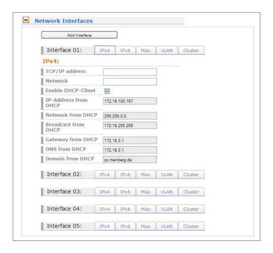
If the DHCP client has been activated, the automatically obtained parameters are shown in the appropriate fields (IPv4 address, netmask, gateway).
