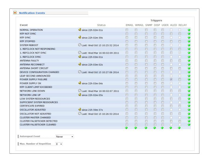
On this page you can set up different notification types for a number of events. This is an important feature because of the nature of a timeserver: running unobserved in the background. If an error or problem occurs, the timeserver is able to notify an administrator by using a number of different notification types.
